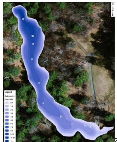
**Deliverables:** ESS will provide the Town with a bathymetry map (in GIS format) with one to two foot contours referenced to an appropriate vertical control such as the dam or spillway.
